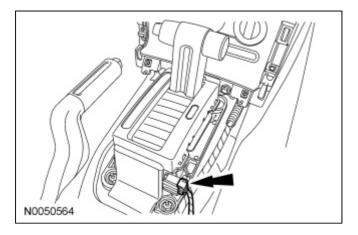
11. Remove the 2 transmission selector lever housing assembly nuts and the 2 transmission selector lever housing assembly screws and carefully lift the transmission selector lever assembly from the vehicle.
