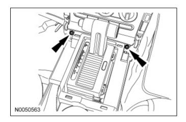
5. Install the 2 nuts into the bottom of the center console.
