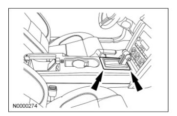
5. Remove the 2 screws and the center console finish panel.
