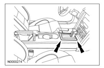
9. **NOTE:** It is necessary to install a new plastic transmission selector lever cable retaining clip prior to installation.
