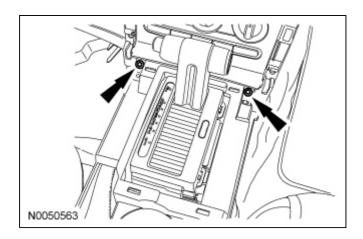
9. Lift up the center console, disconnect the power point electrical connector and remove the center console.
