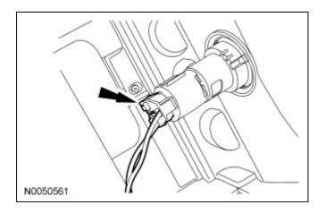
4. Install the 2 screws into the front of the center console.
