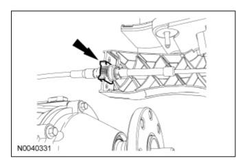
10. Install the transmission selector lever cable onto the selector lever and lock the transmission selector lever cable lock.
