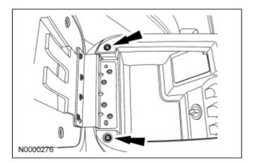
8. Install the center console transmission selector lever trim.
