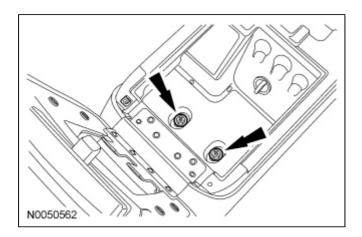
8. Remove the 2 screws from the front of the center console.
