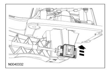
3. Remove the transmission selector lever cable from the bracket and discard the transmission selector lever cable retaining clip.
