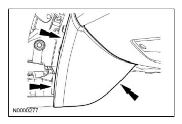
7. Install the center console finish panel and the 2 screws.
