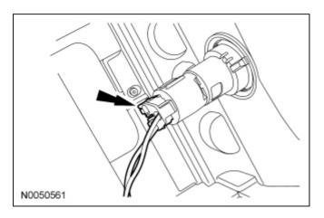
10. Disconnect the transmission selector lever electrical connector.
