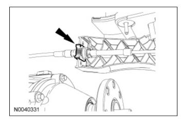
4. Remove the center console transmission selector lever trim.
