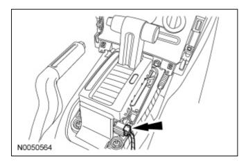
3. Connect the power point electrical connector and install the center console.
