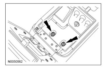
6. Install the driver and passenger side center stack kick panels.
