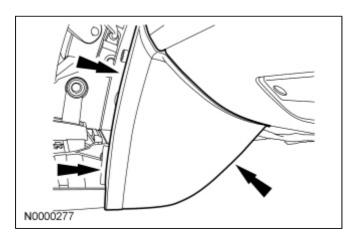
7. Remove the 2 nuts in the bottom of the center console.
